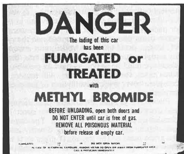
Figure 17. Warning signs on boxcar
