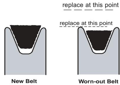
Fan belt wear: thinner, worn belt rides lower in the pulley sheave, which causes fan to run slower. Tightening worn belts does not cure the problem. Replace belts once a year, or whenever the top of a belt is at or below the edge of the pulley sheave.
