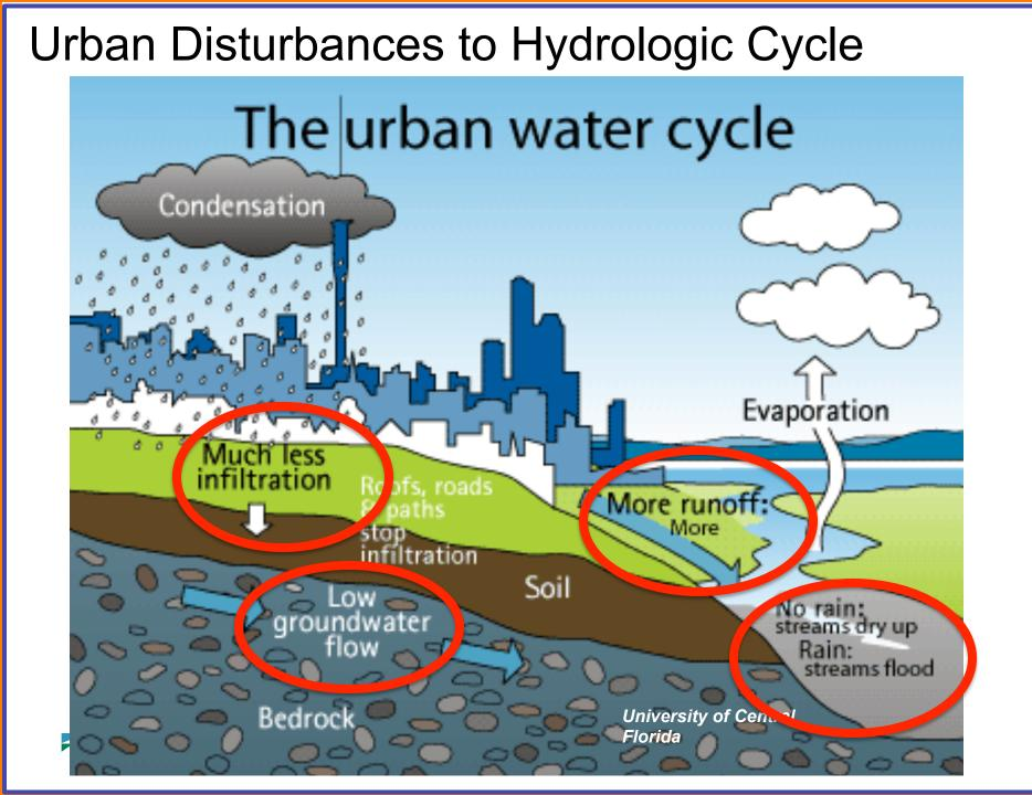
Runoff: *more* Infiltration: *less* Flooding: *more* Baseflow: *less*
