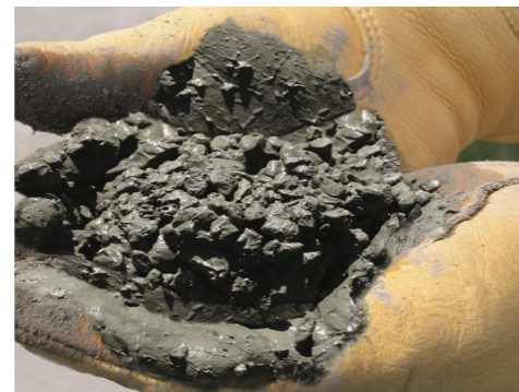
Figures 6.17, 6.18, and 6.19. Mixture consistency (top to bottom): A dry mixture, an ideal mixture, and a wet mixture. (Source: Tennis, Leming, and Akers. 2004.)
