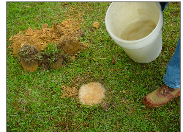
Figure 12.1. Example of infiltration testing.
