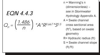
4.4.3. It should first be determined whether the swale will be trapezoidal or triangular; if vegetation other than turfgrass is to be used, a trapezoidal channel is recommended.
