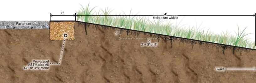
is recommended when there is a single, concentrated flow entering the swale. It serves as a sediment sink for runoff entering the system to prevent clogging of the swale channel and subsequent damage to vegetation.
