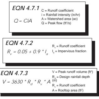
can be used in EQN 4.7.3 to determine the total runoff volume (V).
