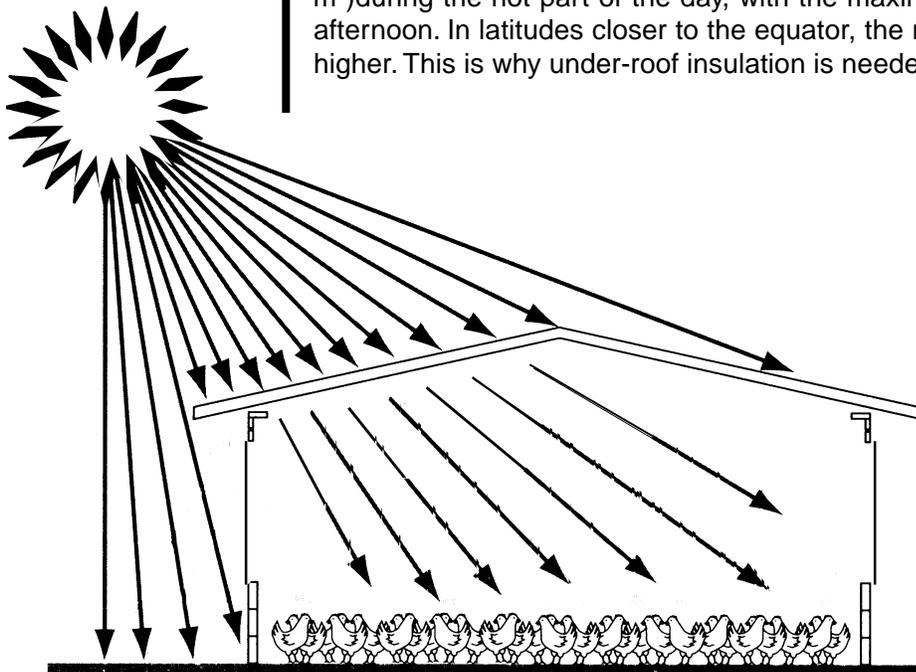
**Metal roof heated by sun to 150°F (66°C) or more radiates large amounts of heat to birds below.**
