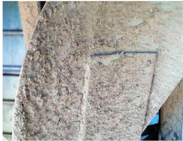
**Keeping tunnel windspeed up to design specification is absolutely essential to getting all of the wind-chill and evaporative cooling you are paying for. If fan belts are worn or dust allowed to built up on fan blades, electric costs stay high but cooling will be severely reduced.**
