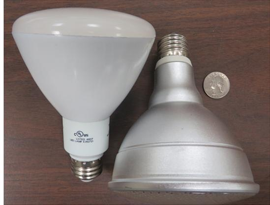
**PAR XX LEDs are floodlight shaped with a curved lens for better light spread. The XX is the number of eighths of an inch the lens is wide. PAR bulbs are most useful in higher wattages as grow lights in open truss ceiling broiler houses. Bulbs pictured above are PAR 30; bulbs at left are PAR 38.**
