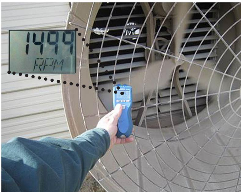
**Just small losses in fan power can mean serious drops in tunnel wind speed – which hurts flock performance. Laser RPM meters offer a handy way to see if tunnel fans are still delivering the needed CFM. RPM meters come in various forms, but all are easy to use. Simply point the laser into the fan from the outside and press the button.**
