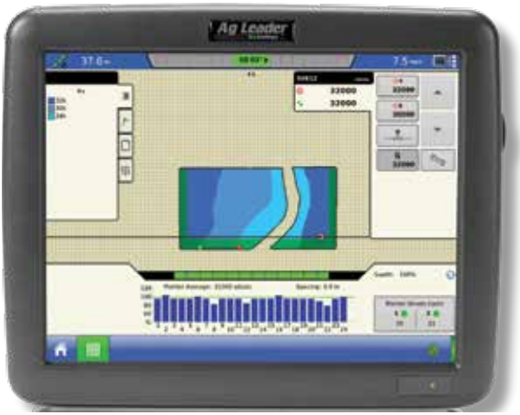
Figure 6. Example display with ASC functionality along with row-by-row population feedback
