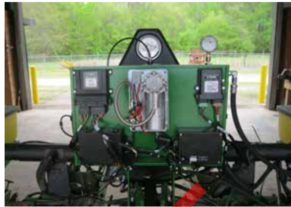
Figure 7. A Trimble air clutch control setup. In the center of this panel is the air compressor with the associated storage (not visible) mounted on the back side. The bottom two black boxes on the left and right are air valve modules used to directly disengage clutches when pressure is applied to the connecting lines. Each air valve module controls up to 4 sections or individual rows. The final component is the ECU on the upper left of the panel. This communicates information between the air valve modules and in-cab display.
